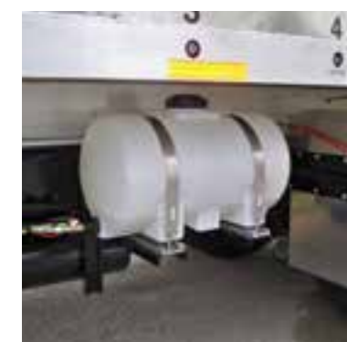
Feed trailers are optioned with cab actuated disinfectant spray systems that douse tires to inhibit the spread of disease from one farm to another.
