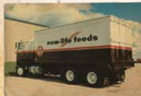
This bag/bulk delivery unit from the mid-1980s used aerodynamic and lightweight FRP/aluminum for a fuel efficient aerodynamic smooth, billboard look.
