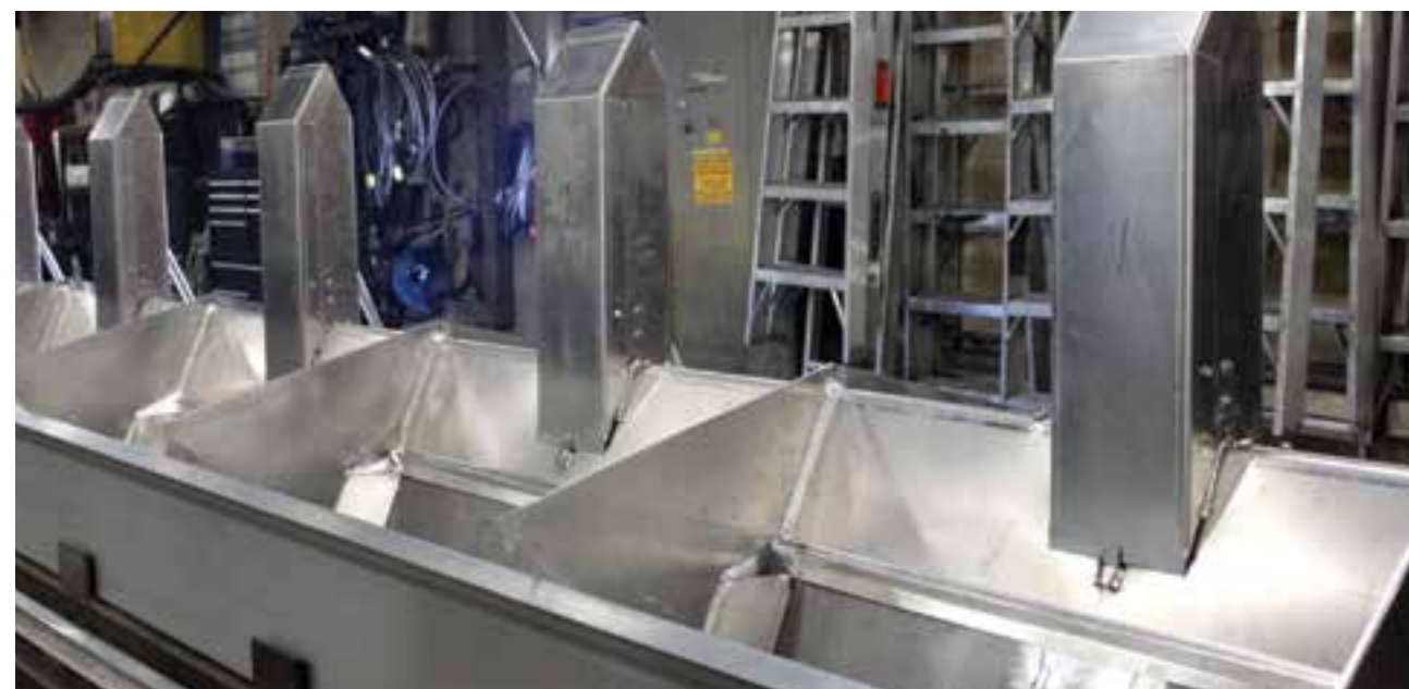
Feed trailers are optioned with cab actuated disinfectant spray systems that douse tires to inhibit the spread of disease from one farm to another.
